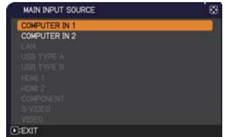
**NOTE** • When FIXED (COMPUTER IN 1) is selected, the MONITOR OUT setting is invalid. ([Operating Guide](#) → [SETUP menu](#))
